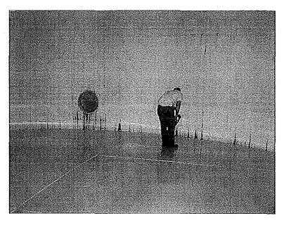
Photo shows the northeast section of the floor. The inspector is checking the DFT of the coating. The white epoxy coating is failing mainly along the sharp edges of the weld seams.
