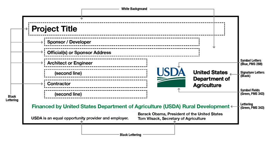
SIGN DIMENSIONS: 1200 mm x 2400 mm x 19 mm (approx. 4' x 8' x ¾") PLYWOOD PANEL (APA RATED A-B GRADE–EXTERIOR)
