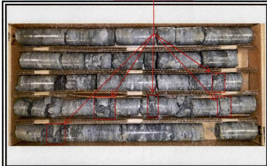
PHOTO #1 – Rock core sample at B-1 from about 7.5 to 17.5 feet below existing grade
