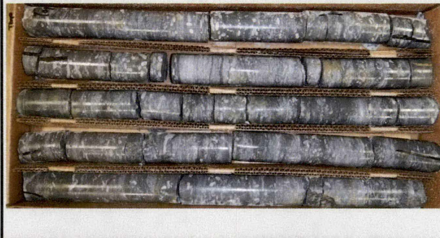
PHOTO #2 – Rock core sample at B-1 from about 17.5 to 27.5 feet below existing grade
