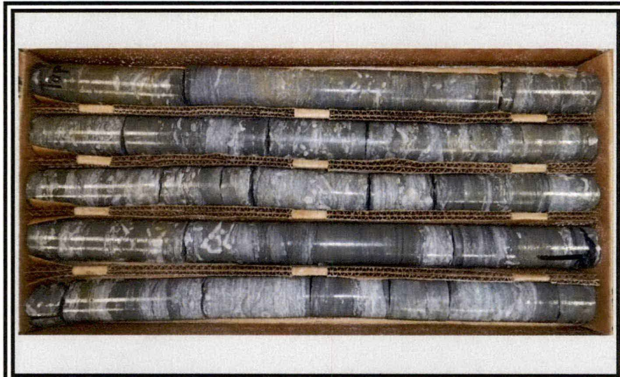
PHOTO #3 – Rock core sample at B-1 from about 27.5 to 37.5 feet below existing grade
