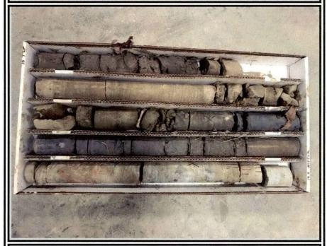
PHOTO #2 - Rock Core sample at B-1 from 10 to 19.5 feet below existing grade
