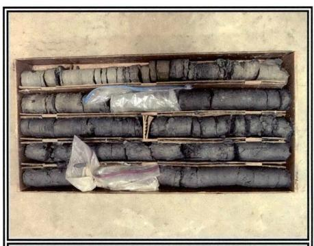
PHOTO #3 – Rock Core sample at B-1A from 19.5 to 29.5 feet below existing grade
