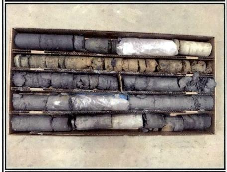
PHOTO #4 – Rock Core sample at B-1A from 29.5 to 39.5 feet below existing grade
