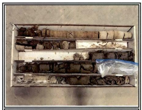
PHOTO #1 - Rock Core sample at B-1 from 2 to 10 feet below existing grade
