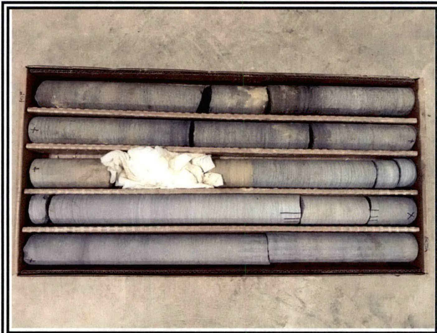
PHOTO #1 – Rock Core sample at B-1 from 14 to 24 feet below existing grade
