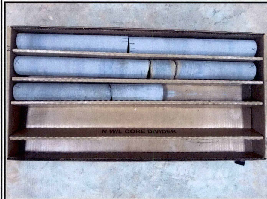
PHOTO #2 – Rock Core sample at B-1 from 24 to 29 feet below existing grade
