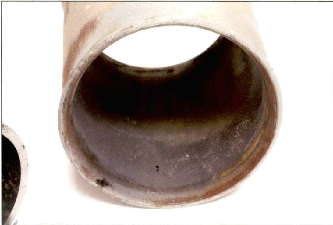
Figure 10. Photograph of the interior of the coupling after disassembly.
