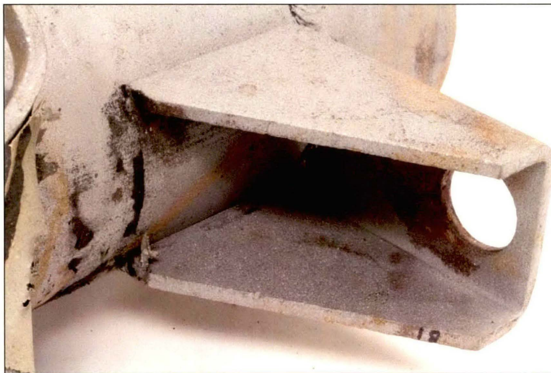
Figure 7. Image of the Lug B1 interior top and exterior bottom locations which were not welded.
