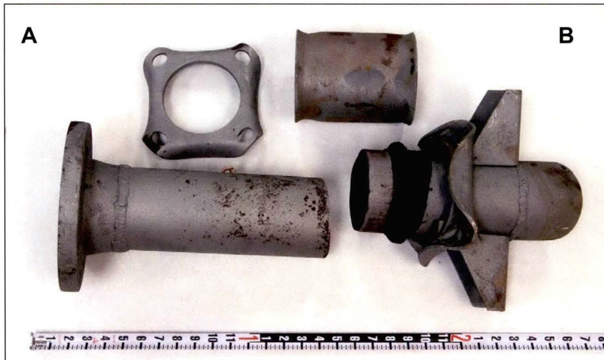
Figure 2. Photograph of the likely bottom of the submitted coupling components.
