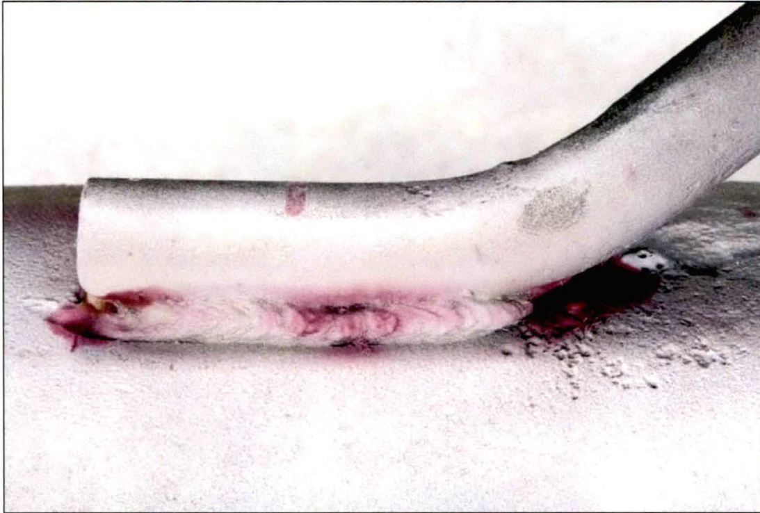
Figure 13. Image of the Rod End A top weld after dye penetrant media had been used during inspection.
