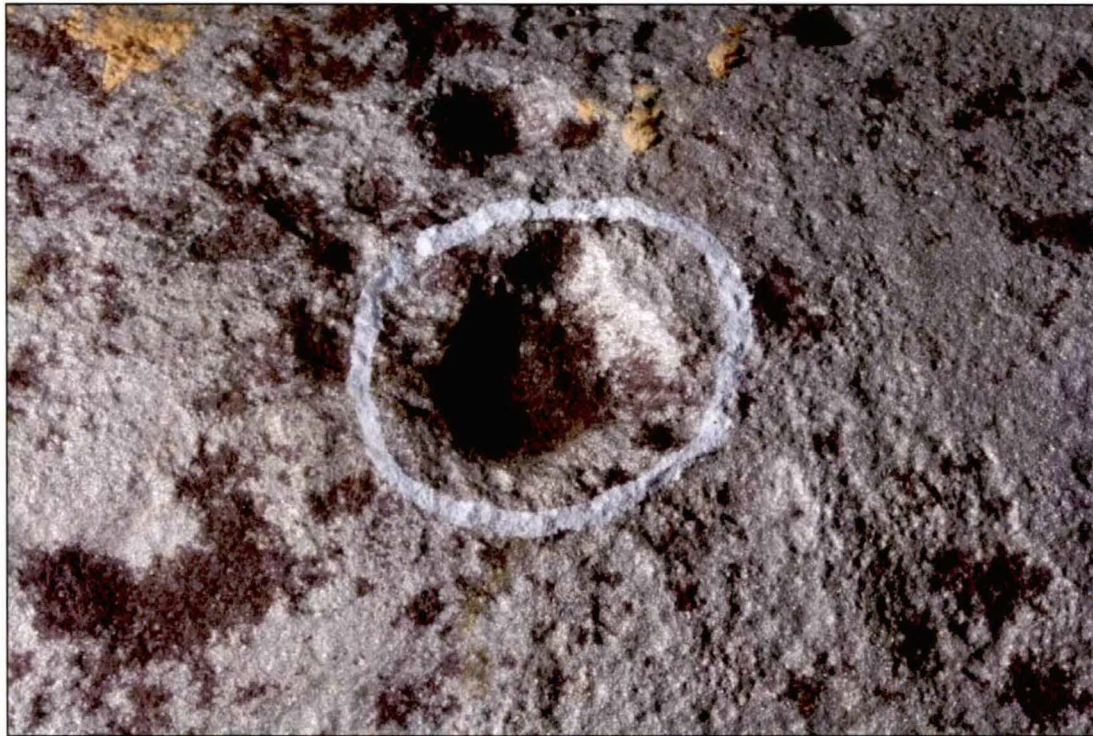
Figure 7. Photograph of a deep corrosion pit on the bottom of the coupling.
