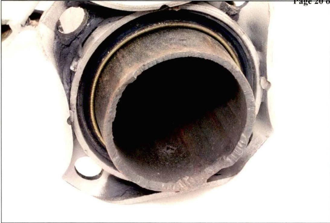
Figure 15. Photograph of the other pipe coupling sample after disassembly.
