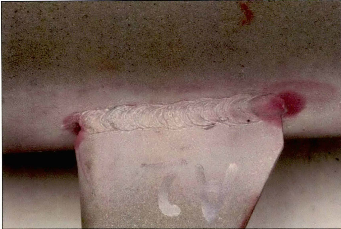
Figure 15. Image of the Lug A2 exterior top weld after dye penetrant media had been used during inspection.
