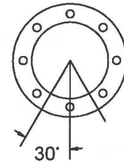
DETAIL A Bolt hole must be aligned with center of tower.
