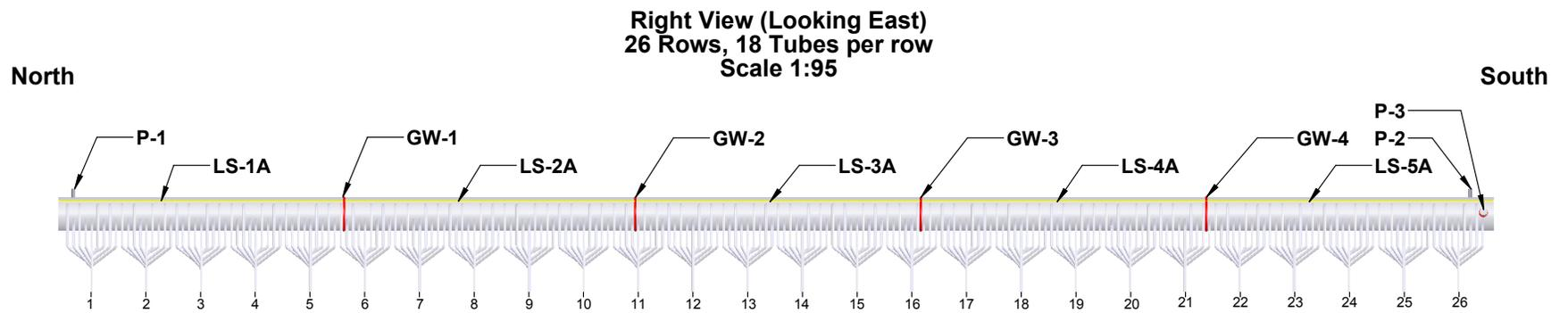
Fig. 1. An overall sketch of the Platen Superheater Inlet header
