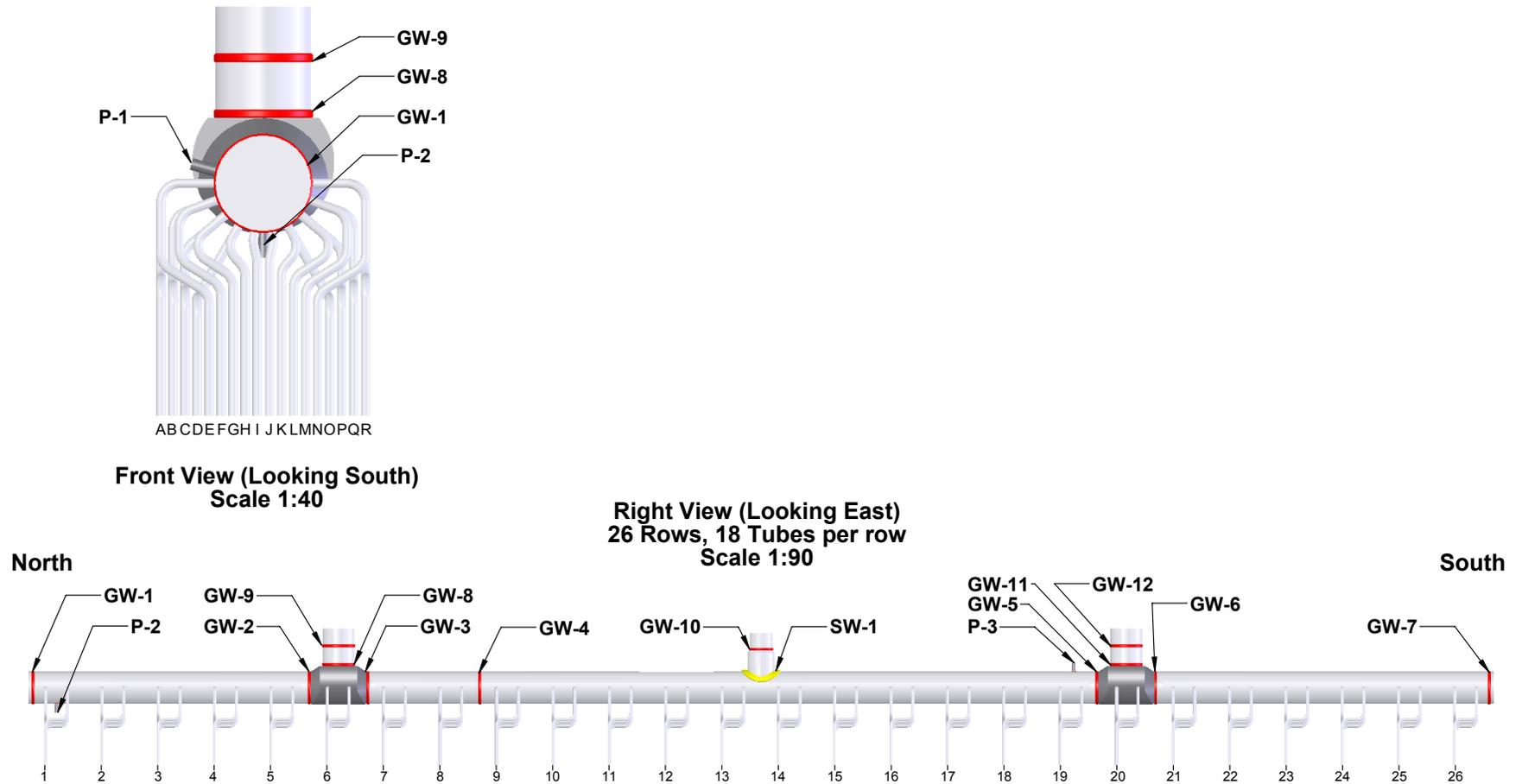
Fig. 15. An overall sketch of the Platen Superheater Outlet header
