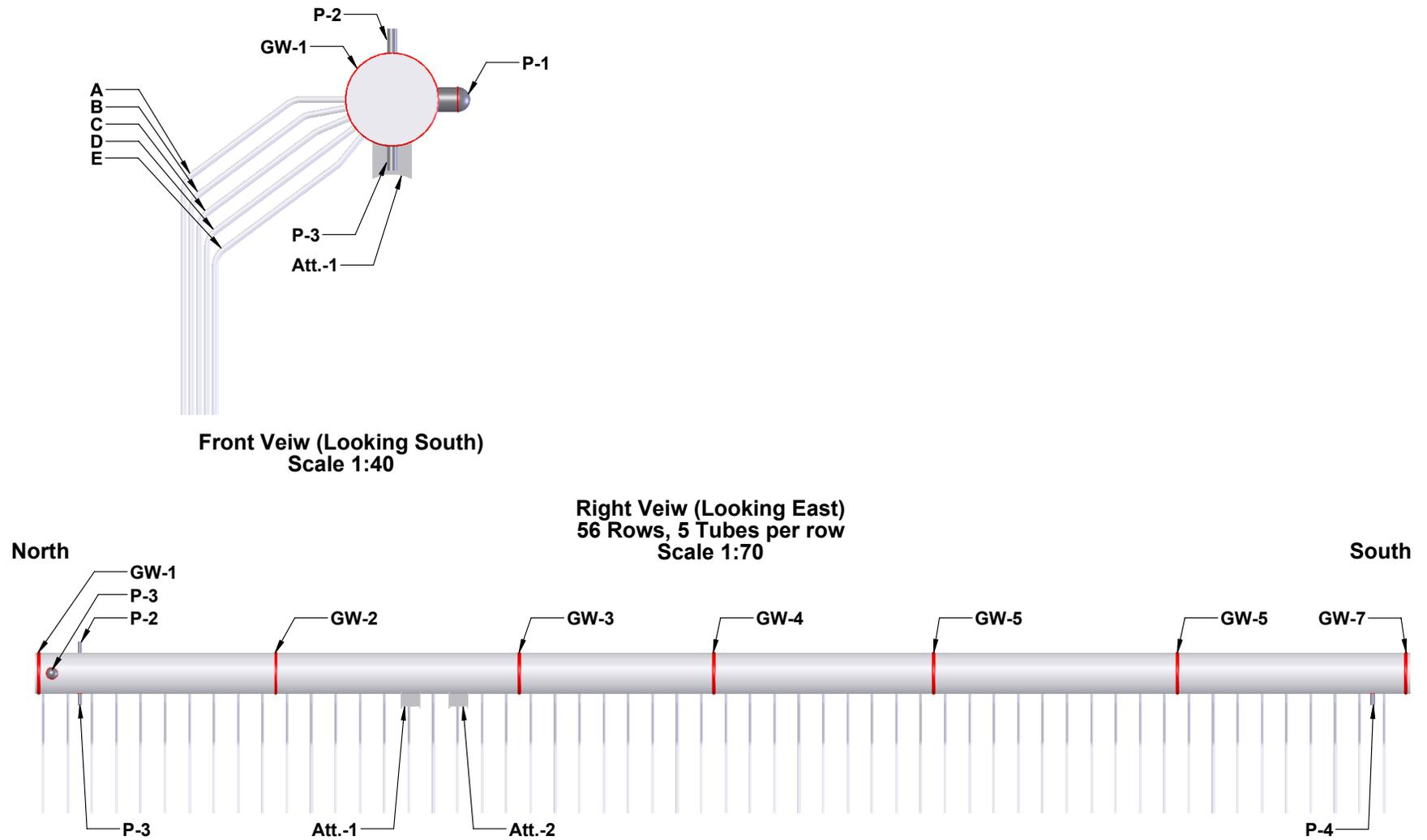
Fig. 48. An overall sketch of the Upper Finishing Superheater Outlet
