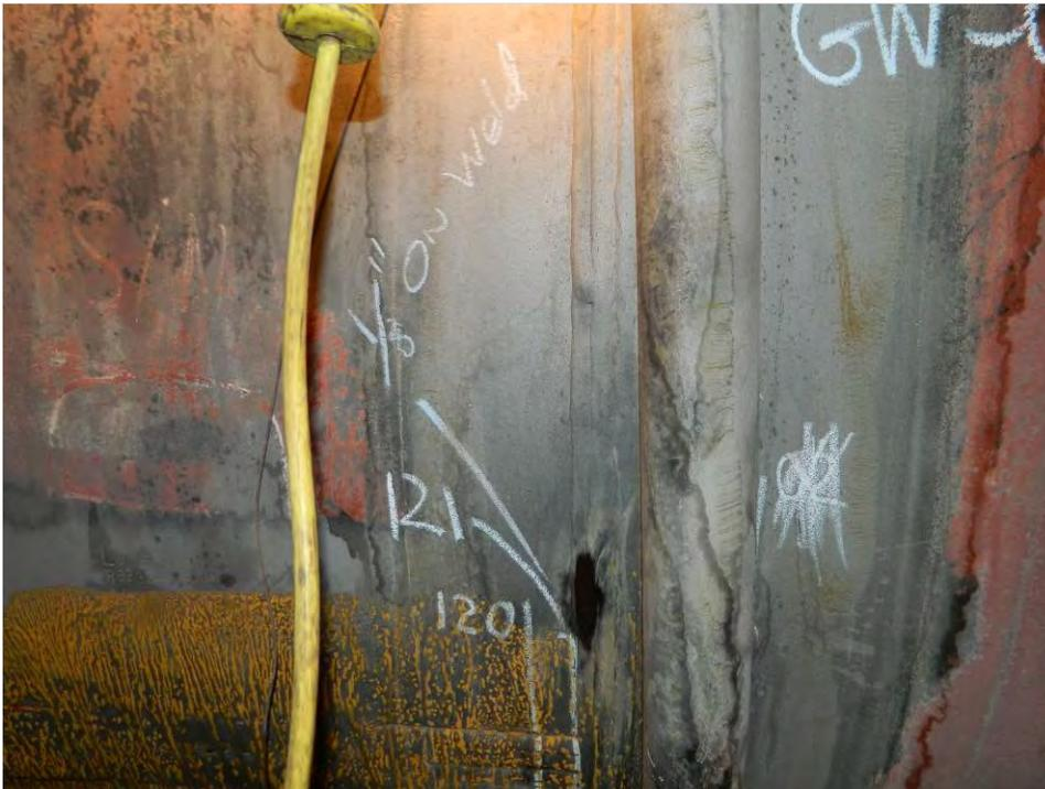
Fig. 90. Photographs of the indications on girth weld No. GW-3 of the LP Reheat Outlet header.
