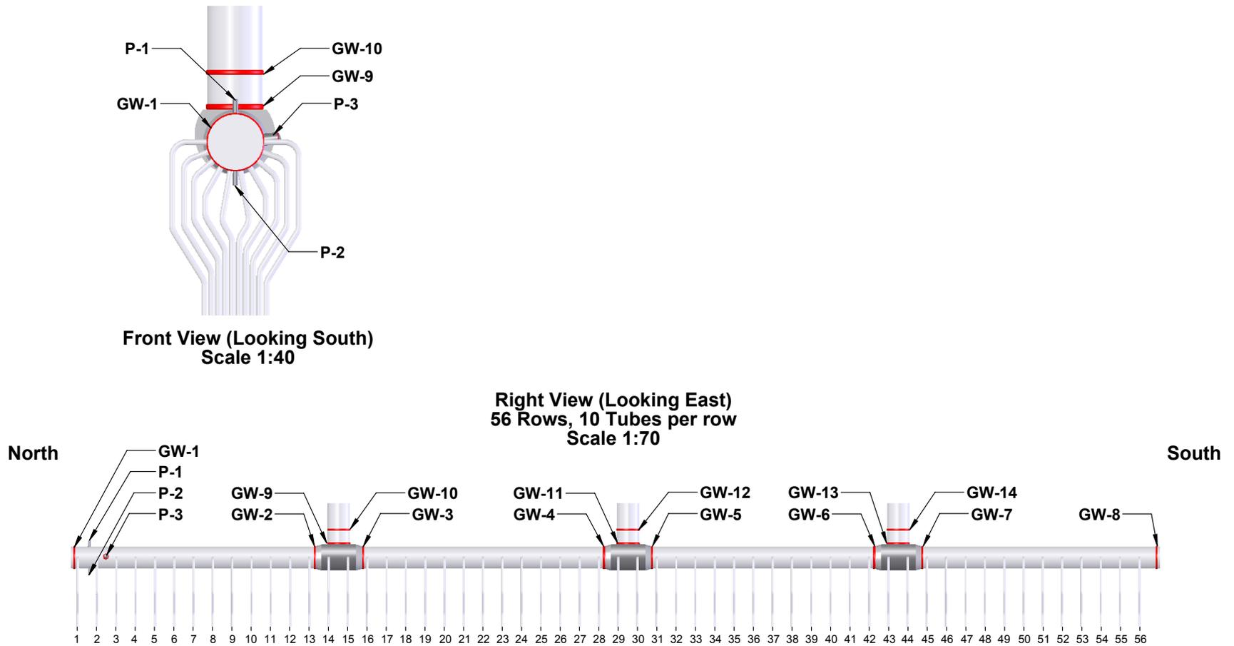
Fig. 31. A sketch of the Finishing Superheater Inlet header
