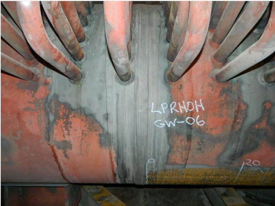
Fig. 86. Photographs of girth weld Nos. GW-5 and GW-6 on the LP Reheat Outlet header
