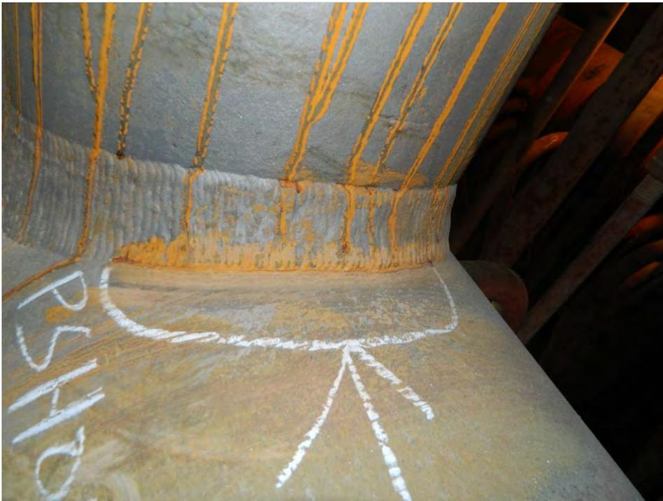
Fig. 22. Photographs of the indication on saddle weld No. SW-1 of the Platen Superheater Outlet header.
