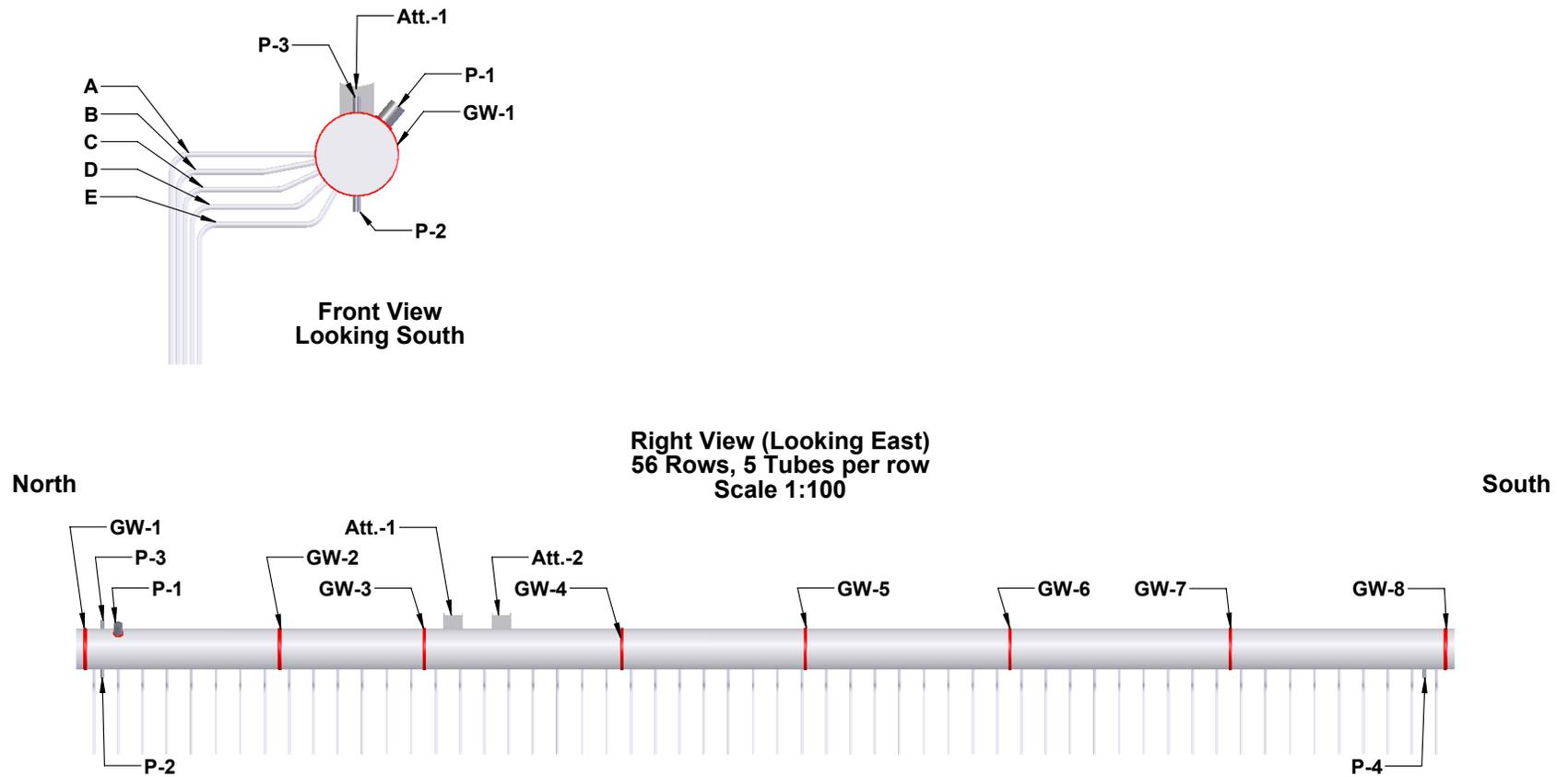
Fig. 49. An overall sketch of the Lower Finishing Superheater Outlet
