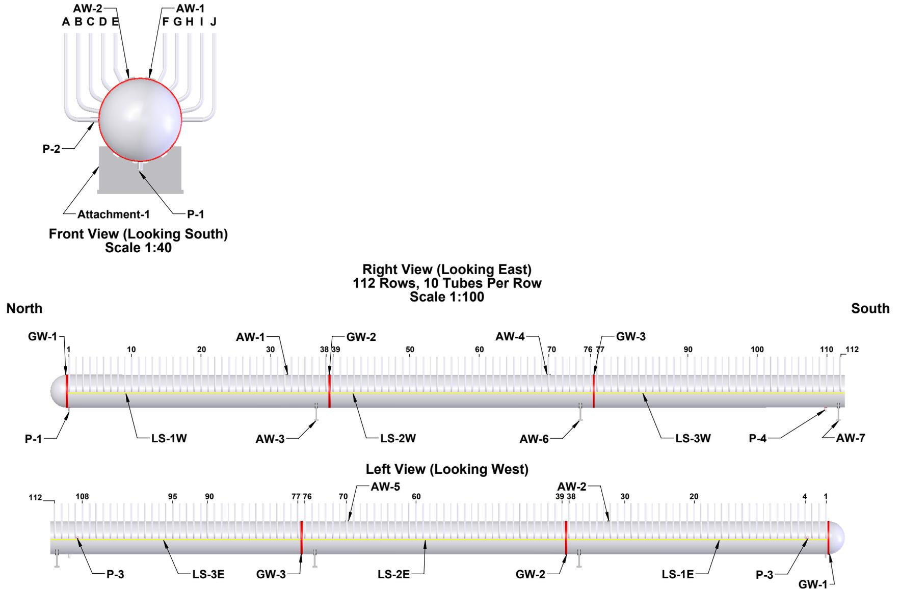
Fig. 72. An overall sketch of the High-Pressure Reheat Outlet header
