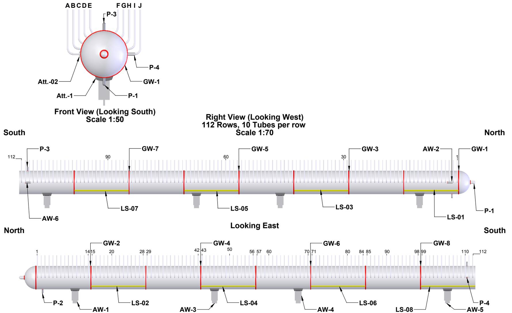
Fig. 84. An overall sketch of the Low-Pressure Reheat Outlet header
