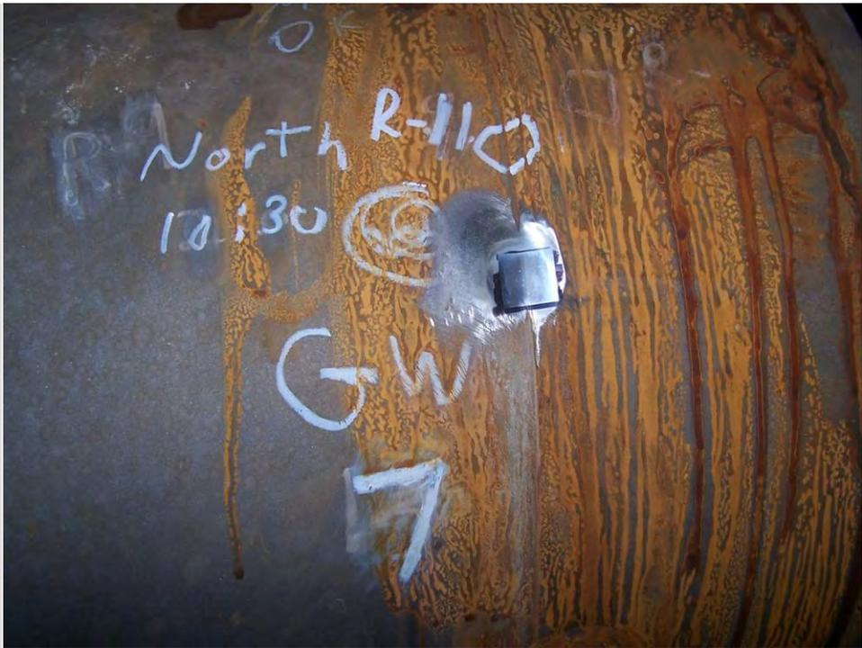
Fig. 17. Photographs of the inspection locations on the Platen Superheater Outlet header.
