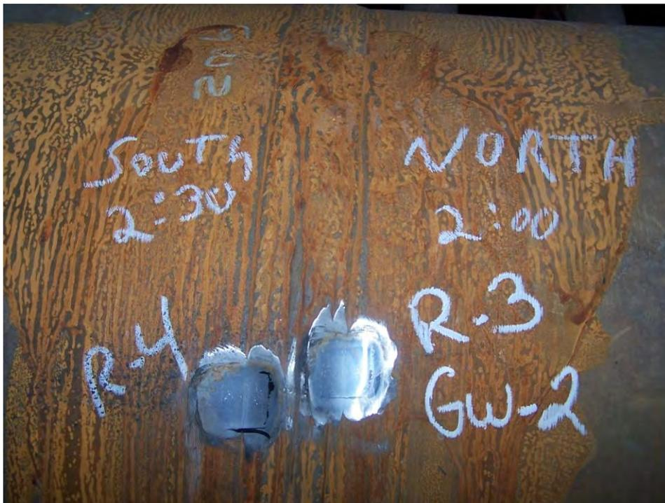
Fig. 3. Photographs of the inspection locations on the Platen Superheater Inlet header.
