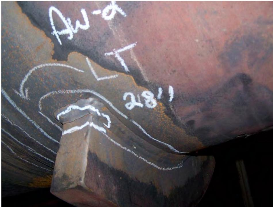
Fig. 95. Photographs of indications in attachment weld No. AW-2 on the High-Pressure Reheat Outlet header.
