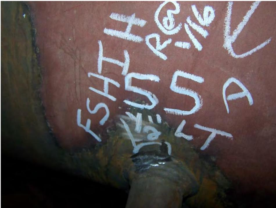
Fig. 34. Photograph of indication before and after removal in tube stub 55A on the Finishing Superheater Inlet header.
