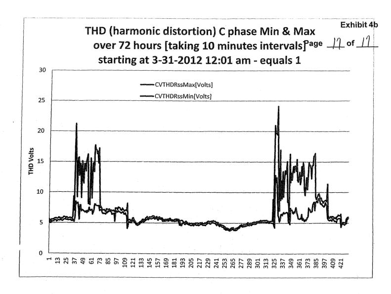
While there is no national standard dictating THD limits on systems, there are recommended values for acceptable harmonic distortion. IEEE Std 519, "RECOMMENDED PRACTICES AND REQUIREMENTS FOR HARMONIC CONTROL IN ELECTRICAL POWER SYSTEMS" provides suggested harmonic values for power systems:
