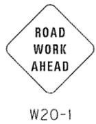
"ROAD WORK AHEAD" SIGN TO BE PLACED ALONG US 42 THROUGHOUT THE DURATION OF THE CONSTRUCTION WITHIN US 42 RIGHT OF WAY, AT APPROPRIATE LOCATIONS TO WARN THE PUBLIC AHEAD OF THE CONSTRUCTION ACTIVITY AREA.
