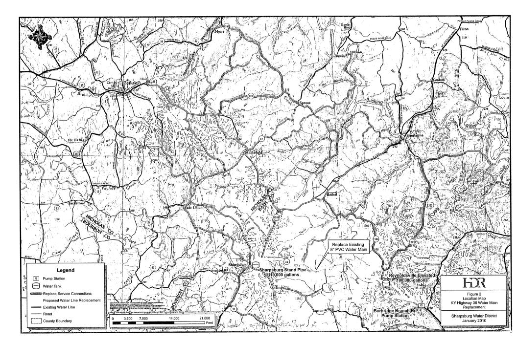
Portions of the work within the state highway rights-of-way will require Encroachment Permits from the Kentucky Transportation Cabinet, Department of Highways. Encasement pipe will be installed at locations where the water main crosses state highways.
