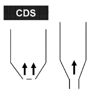
Lower velocity in upper part of reactor, acceleration through venturi
