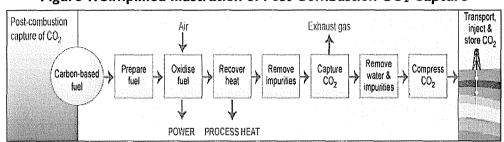
Figure 1. Simplified Illustration of Post-Combustion CO<sub>2</sub> Capture
