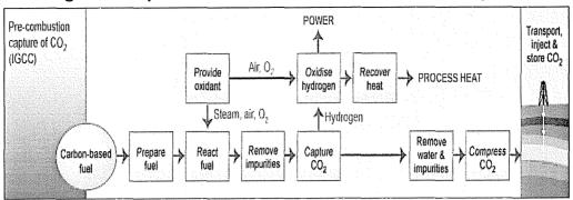
Figure 2. Simplified Illustration of Pre-Combustion CO<sub>2</sub> Capture
