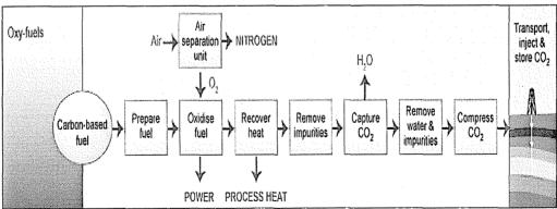
Figure 3. Simplified Illustration of Oxy-Fuel CO<sub>2</sub> Capture
