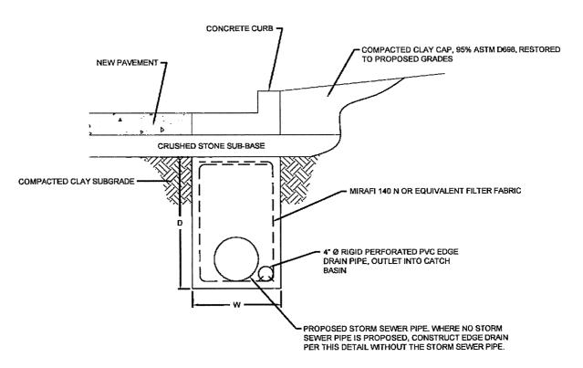
W = TRENCH WIDTH. 12" MINIMUM WHERE 4" DIA. PERFORATED DRAIN PIPE ONLY, WITH NO STORM SEWER. STORM PIPE DIAMETER PLUS 2 FEET WHERE STORM SEWER IS PROPOSED.
