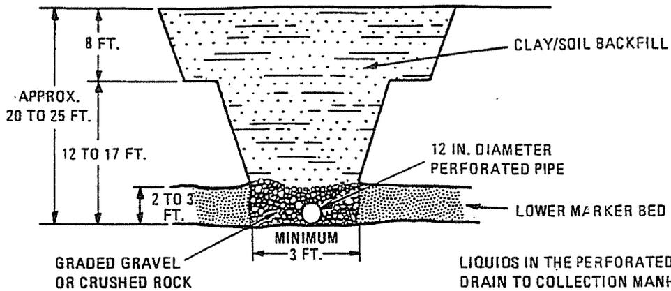
LIQUIDS IN THE PERFORATED PIPE WILL DRAIN TO COLLECTION MANHOLE (SEE DETAIL BELOW) AND PUMPED INTO A STORAGE TANK FOR TREATMENT AND DISPOSAL.
