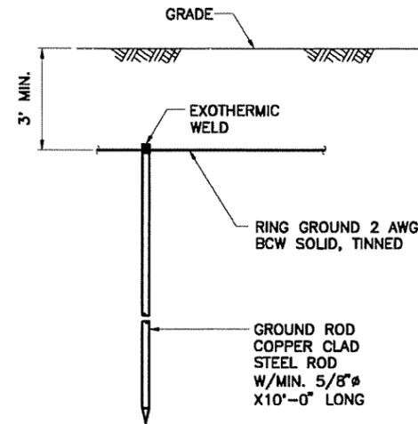
1. GROUND ROD SHALL BE DRIVEN VERTICALLY, NOT TO EXCEED 45 DEGREES FROM THE VERTICAL.
