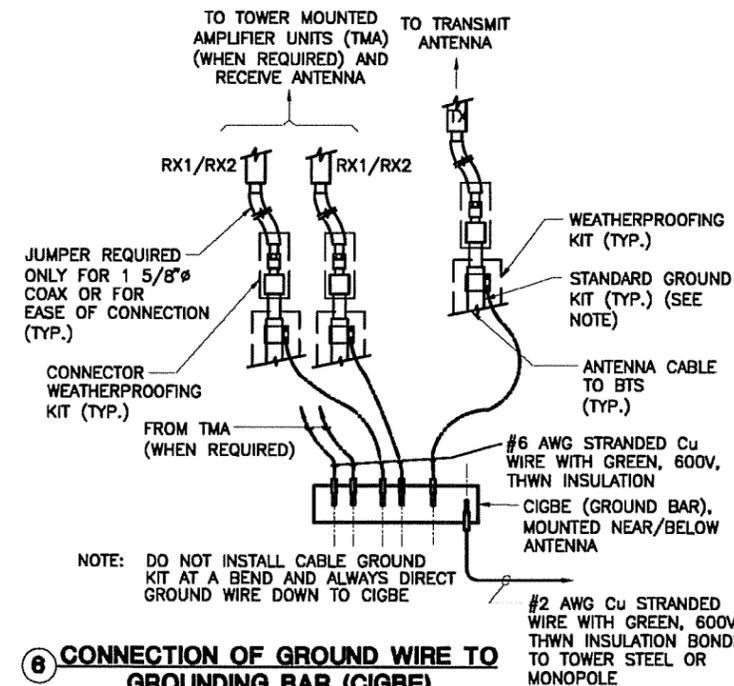
**6 CONNECTION OF GROUND WIRE TO GROUNDING BAR (CIGBE) TOWER/MONOPOLE**
