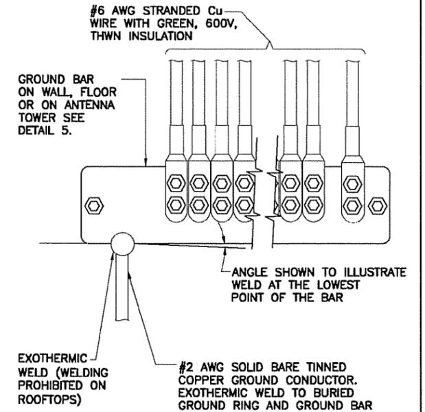
**4 INSTALLATION OF GROUND WIRE TO GROUND BAR DETAILS**
