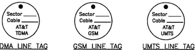
TO PROVIDE ADDITIONAL IDENTIFICATION EACH RF CABLE SHALL BE IDENTIFIED WITH A METAL TAG MADE OF STAINLESS STEEL OR BRASS AND STAMPED WITH THE SECTOR, CABLE NUMBER, AND "AT&T" TO IDENTIFY AT&T MOBILITY CABLES. THE ID MARKING LOCATIONS SHOULD BE AS PER "CABLE MARKING LOCATIONS TABLE". THE TAG SHOULD BE ATTACHED WITH CORROSION PROOF WIRE AROUND THE CABLE. PREFERRED TAG LABELING SHOULD BE AS SHOWN ABOVE "TDMA LINE TAG", "GSM LINE TAG" AND "UMTS LINE TAG".
