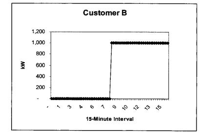
As can be seen from these two graphs, Customer A's load is up when Customer B's load is down, and Customer B's load is up when Customer A's load is down. When the loads for these two customers are aggregated (or *convolved*), the combined load for the two customers flatten out as follows:
