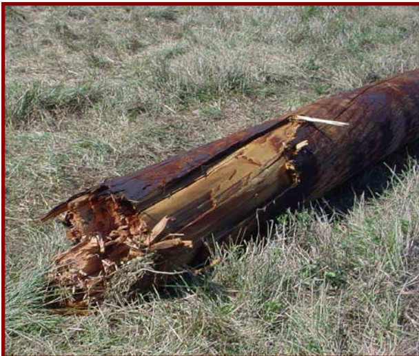
LG&E pole snapped by the 2008 wind storm PSC photo
