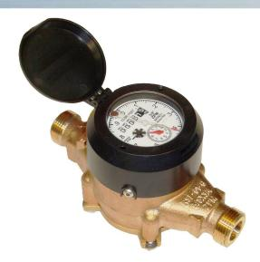
earth magnets eliminate slipping and uncoupling to increase overall accuracy. The magnet is connected to a gear train which translates the impeller's rotation into volume totalization displayed on the register dial face.
