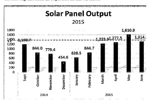
The panels have generated anywhere from 454 kWh to 1610 kWh in a month since they have been in production. The average has been 1016.8 kWh per month. June typically would have been a higher production month than May if not for the cloudiness caused by all the rain.
