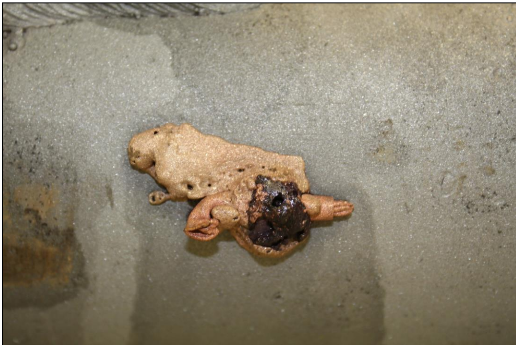
Figure 10. Image of the remainders of an additional piece, which had been welded then cut off, present on Side A of the assembly.
