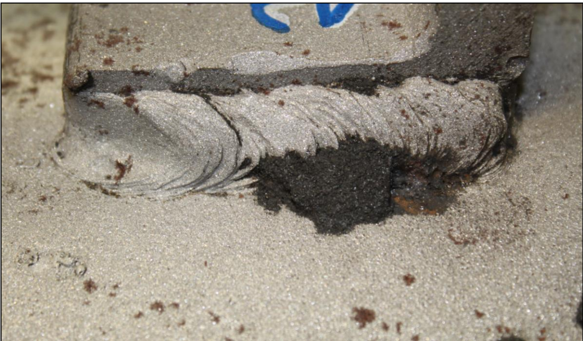
Figure 6. Image of the Lug A3 exterior top weld which exhibited substantial fusion except for some spatter and undercut.
