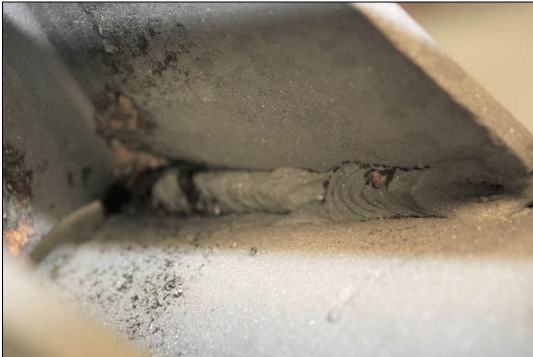
Figure 9. Image of the Lug B1 interior bottom weld which exhibited substantial fusion except for some porosity and spatter.
