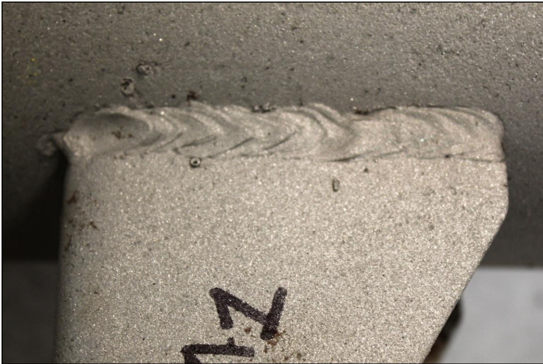
Figure 5. Image of the Lug A1 exterior top weld which exhibited substantial fusion except for some porosity and spatter.
