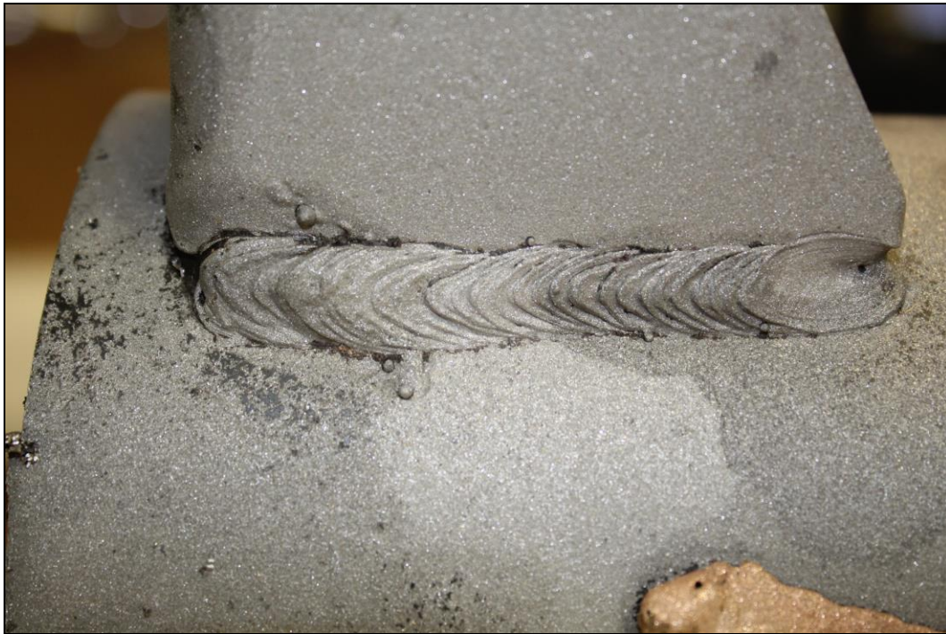
Figure 5. Image of the Lug A2 exterior top weld which exhibited substantial fusion except for some arc burn, porosity, undercut, and spatter.
