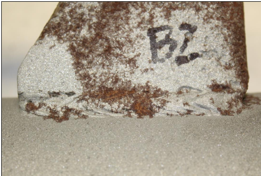
Figure 7. Image of the Lug B2 exterior top weld which exhibited substantial fusion except for some undercut, and porosity. Pitting corrosion damage was observed.
