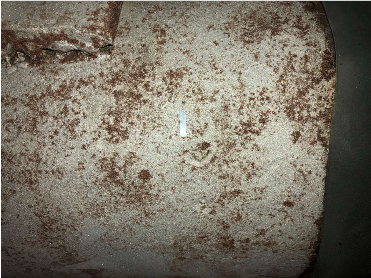
Figure 11 Pipe B Pits
