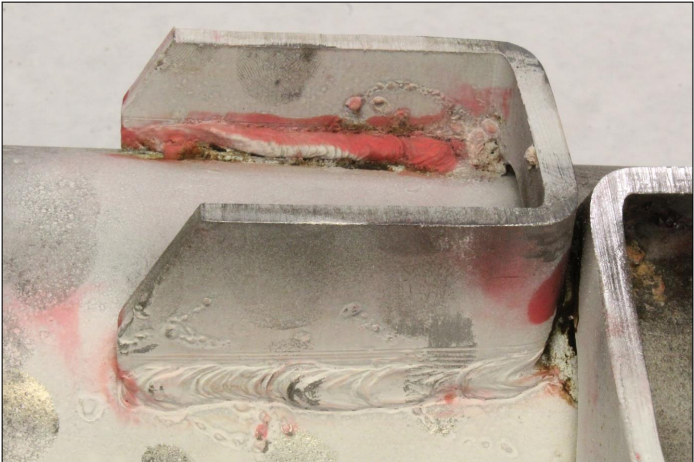
Figure 12. Image of the Lug B1 exterior top welds after dye penetrant media had been used during inspection.
