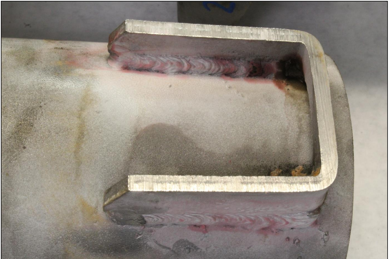
Figure 11. Image of the Lug A1 exterior top welds after dye penetrant media had been used during inspection.
