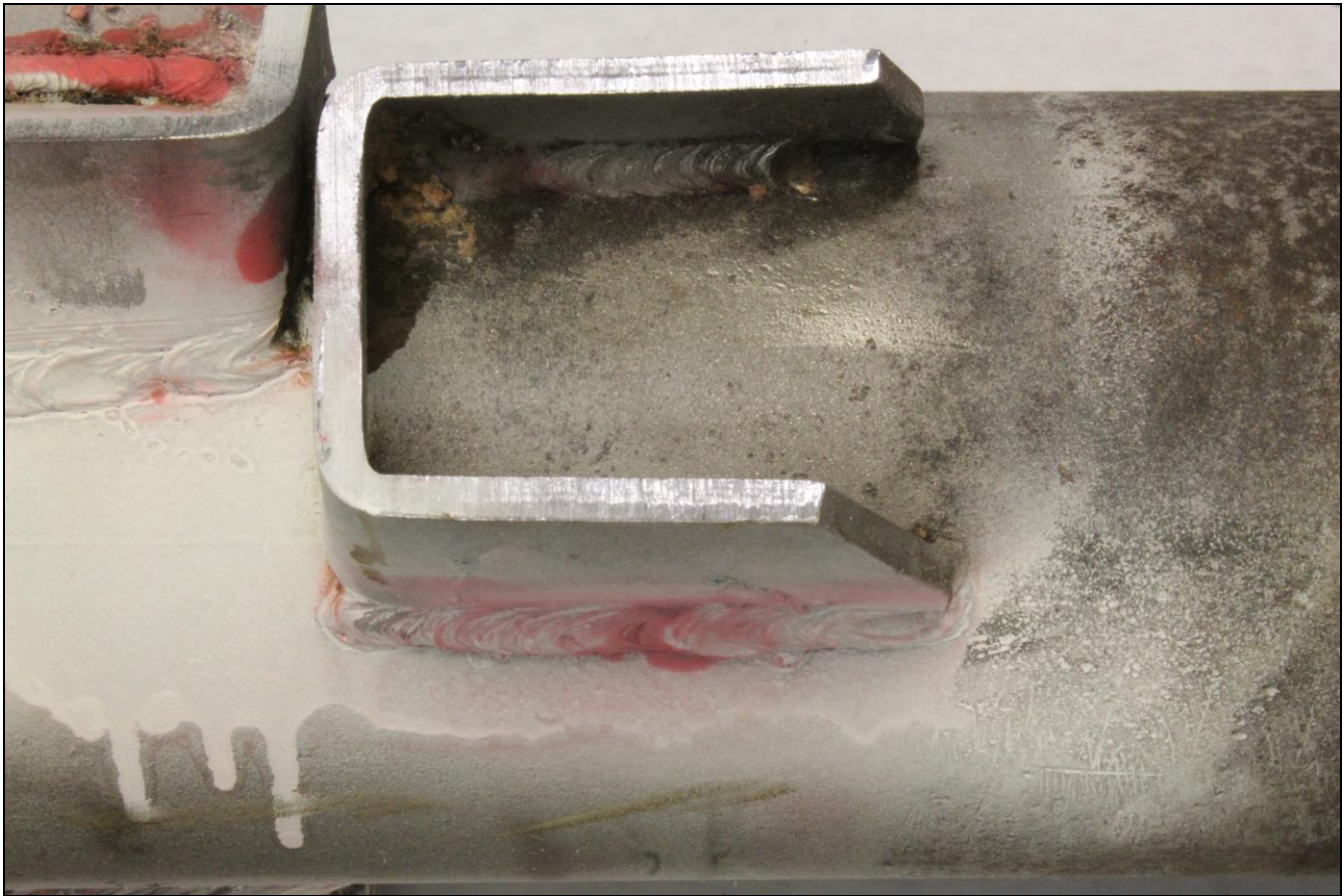
Figure 9. Image of the Lug B2 exterior top welds after dye penetrant media had been used during inspection.
