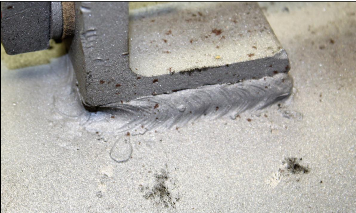
Figure 9. Image of the Lug B3 exterior top weld which exhibited substantial fusion except for some arc burn, porosity, spatter and undercut.
