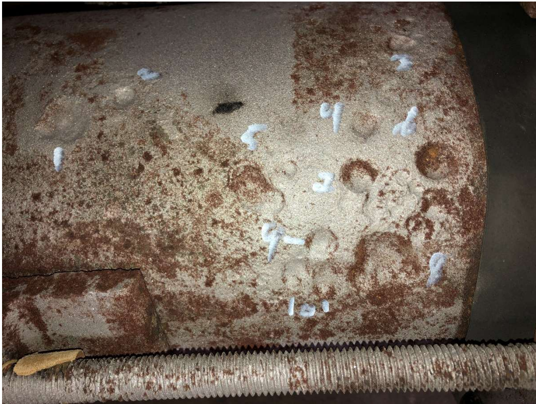
Figure 8 Pipe A Pits
