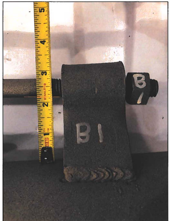
Figure 14- Lug B1, 2-3/16 inches from pipe
