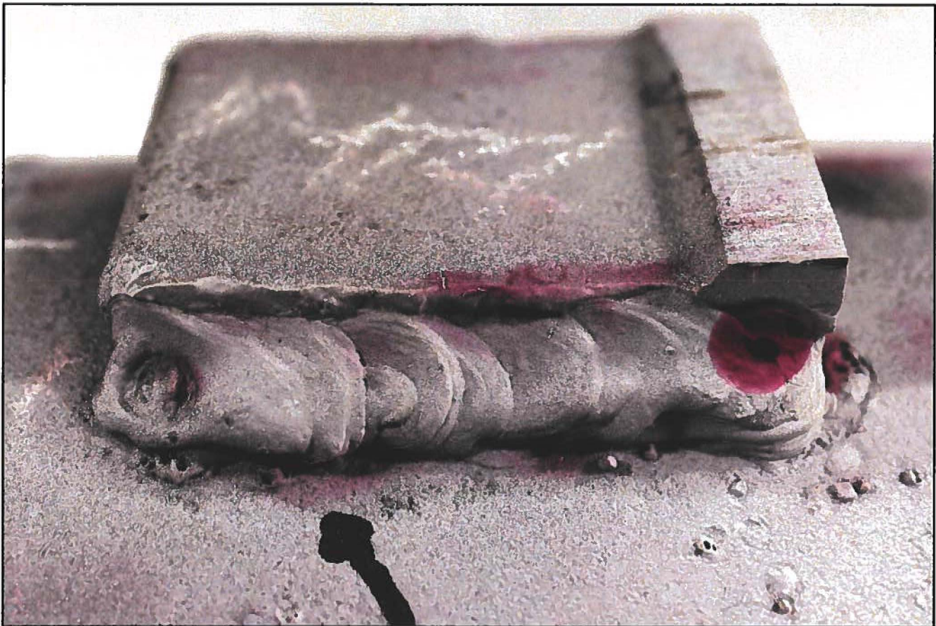
Figure 16. Image of the Lug B2 exterior top welds after dye penetrant media had been used during inspection.
