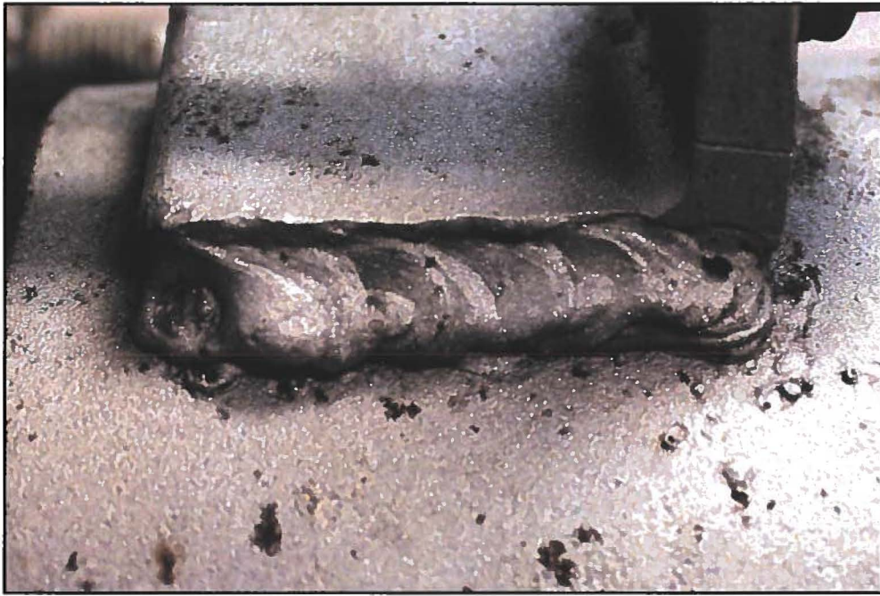
Figure 9. Image of the Lug B6 exterior top weld which exhibited substantial fusion except for some arc burn, porosity, spatter and undercut.
