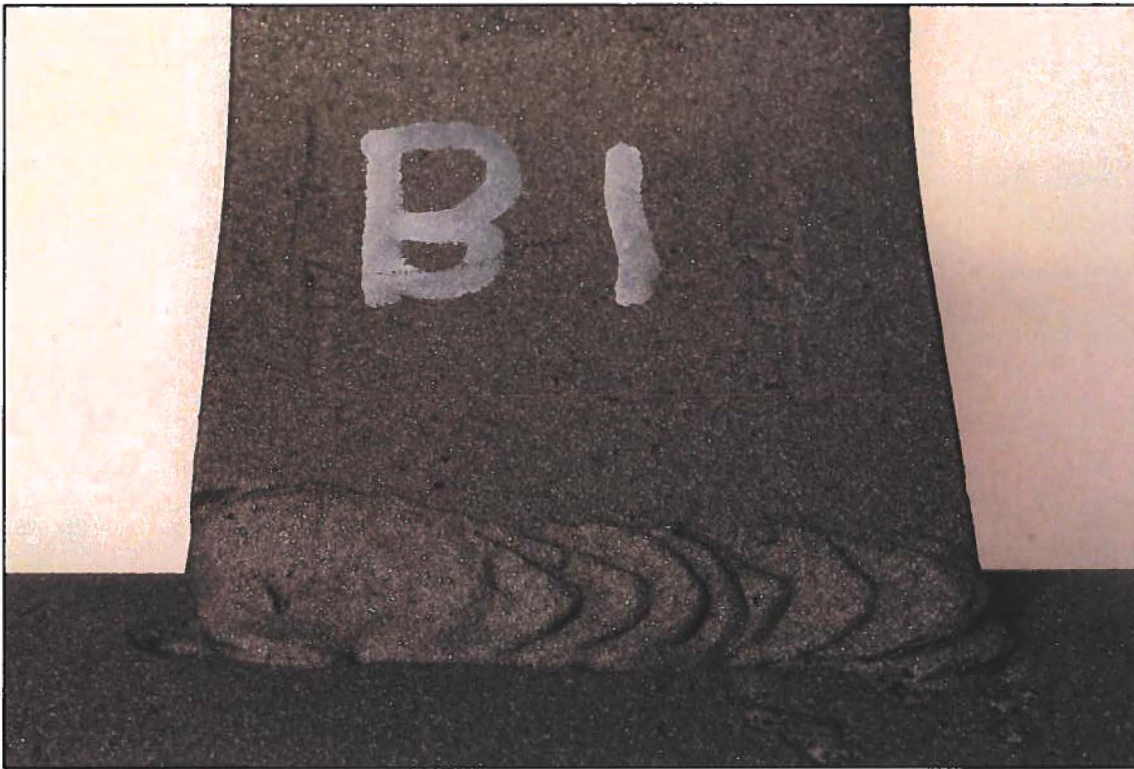
Figure 5. Image of the Lug B1 exterior top weld which exhibited substantial fusion except for some overlap, spatter, arc strike and porosity.
