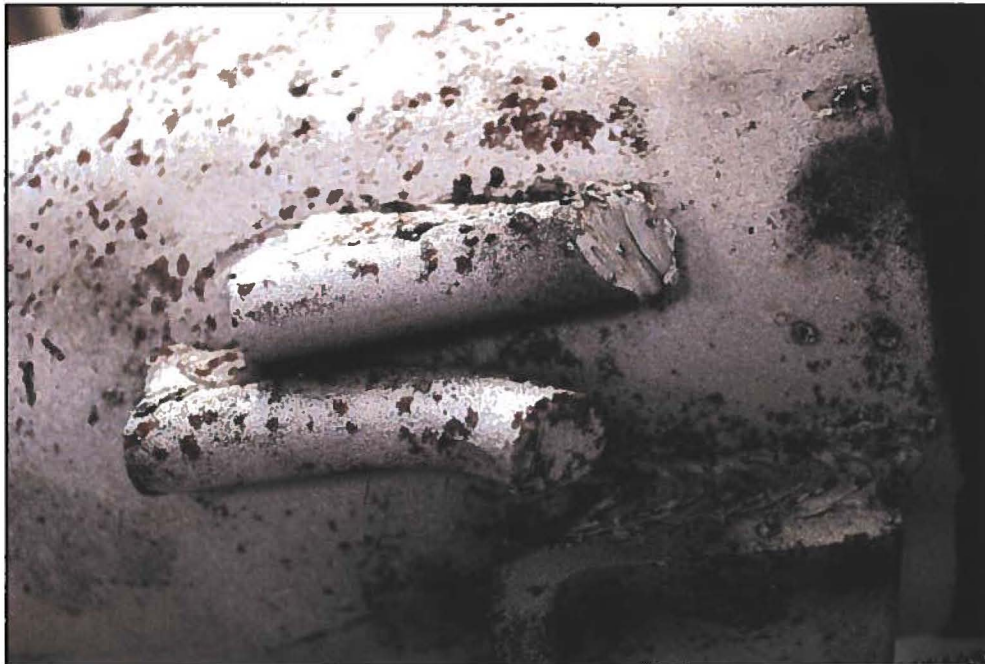
Figure 12. Image of the remainders of additional rods, which had been welded then cut off, present on Side B of the assembly.
