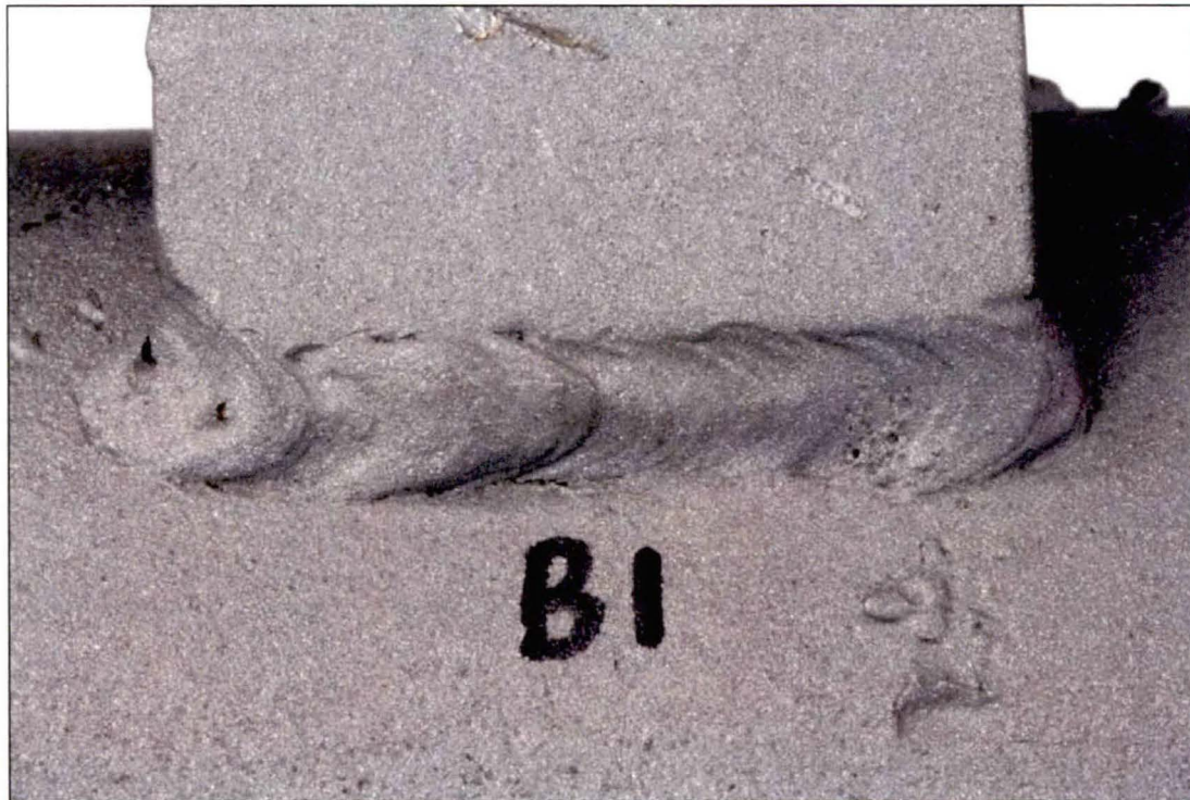
Figure 6. Image of the Lug B1 exterior top weld which exhibited minimal porosity.
