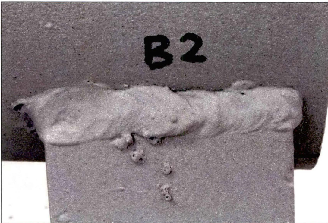
Figure 9. Image of the Lug B2 exterior top weld which exhibited substantial fusion except for some overlap and spatter.
