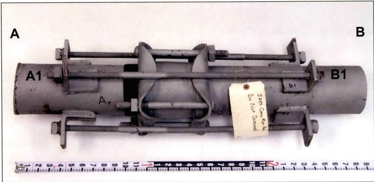
Figure 1. Photograph of the top of the submitted coupling sample. Three attachment rods were affixed with angle iron lugs. Lugs A1 and B1 are identified.
