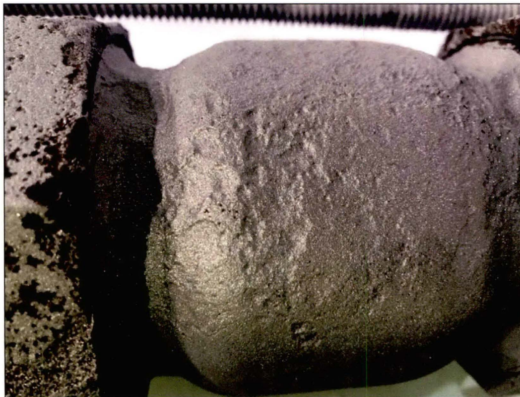
Figure 9- Corrosion Coupling Body version 5.1 (12/06/2018)
