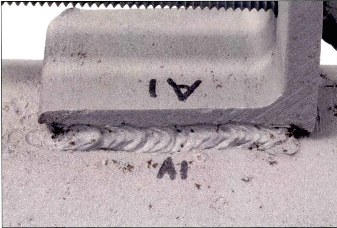
Figure 5. Image of the Lug A1 left weld which exhibited substantial fusion. Some porosity was apparent.
