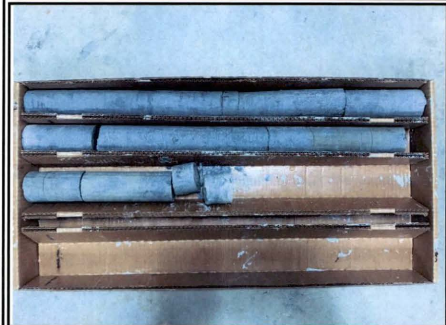
PHOTO #2 – Rock Core sample at B-1 from 39 to 44 feet below existing grade
