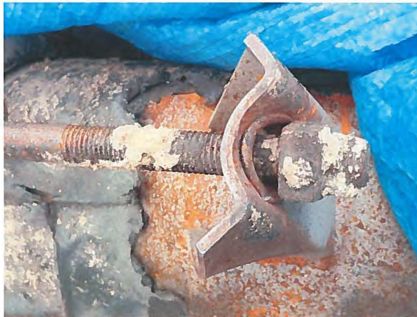
Figure 39. Bracket distortion from compression overload. Note absence of washer
