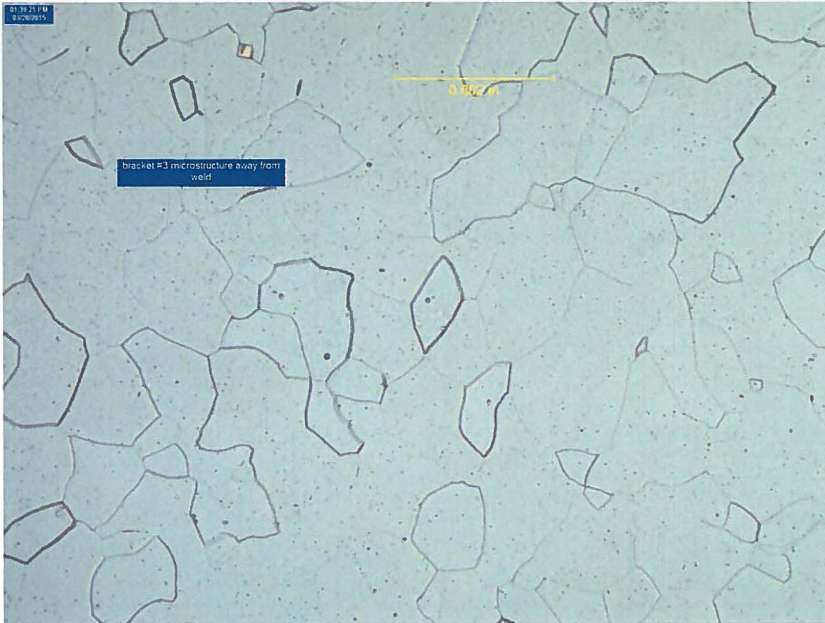
Figure 31. Microstructure of bracket material away from weld
