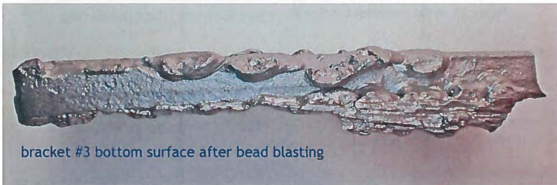
Figure 12. D side bracket #3, leg #2 after glass bead blasting
