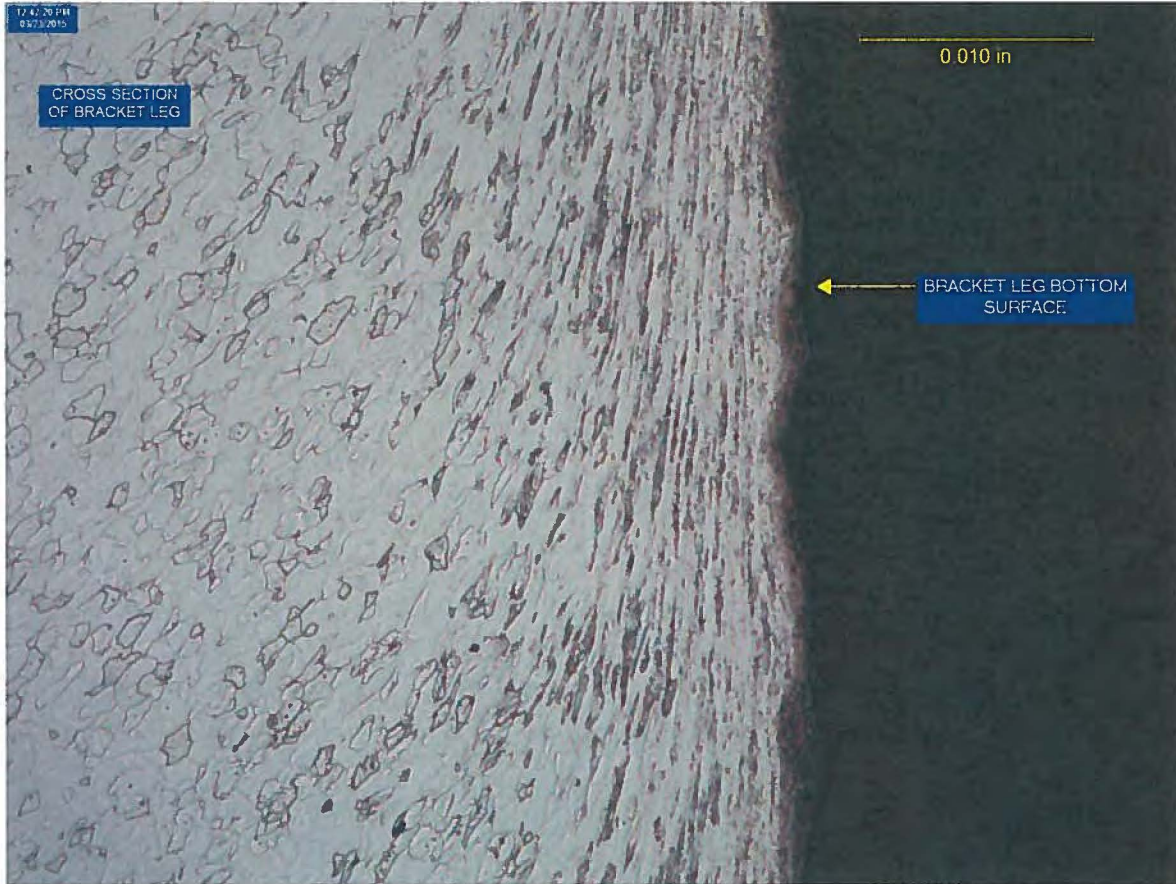
Figure 28. D side bracket #3 cross section of bottom of leg
