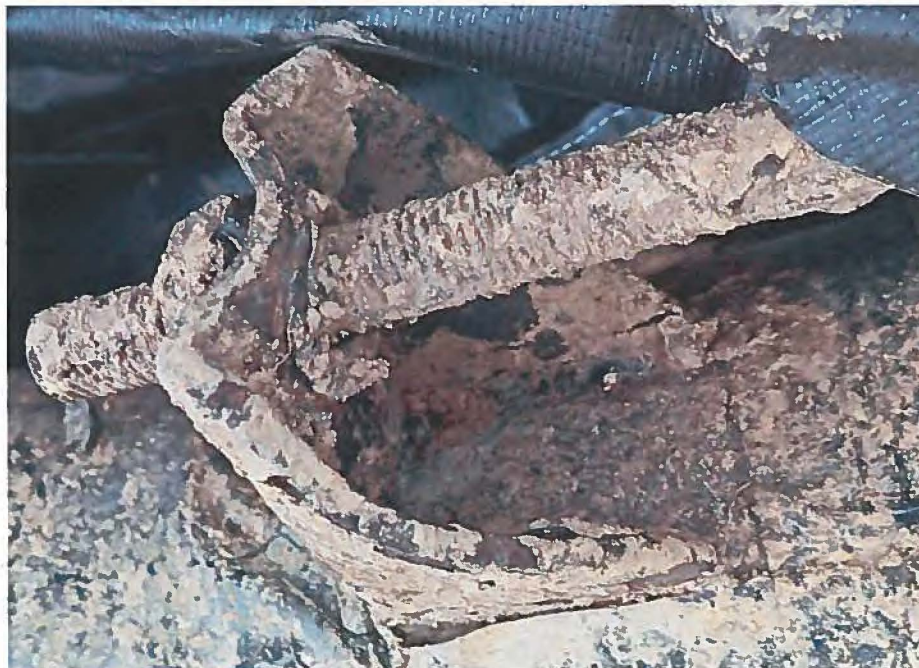
Figure 35. 8" bracket before blast cleaning. Bracket compression surface has deformed under load.
