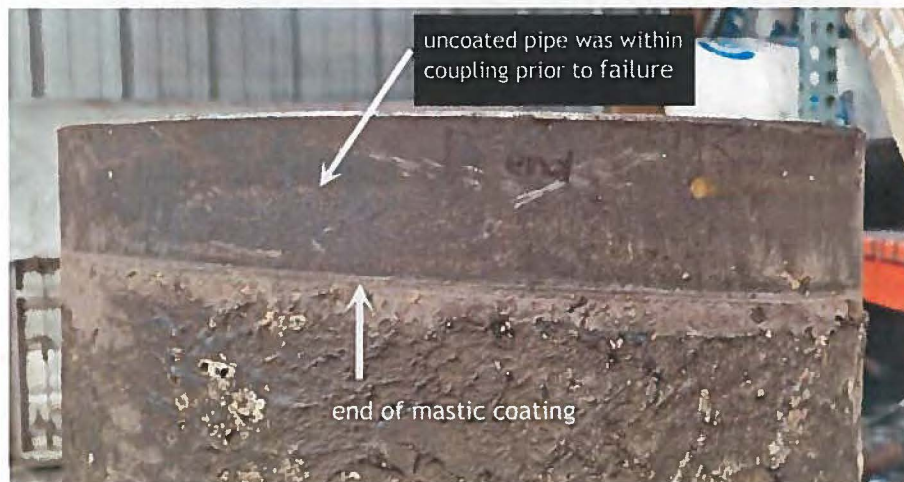
Figure 21. D end of pipe, this end was inserted into coupling
