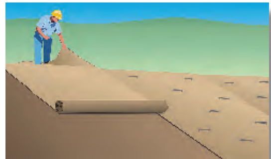
Install blankets and mats vertically on long slopes. Trench and staple top section, overlap sides 3 to 6 inches. Follow manufacturer’s directions regarding stapling and slope limitations. For areas that will be mowed, specify blankets without plastic netting or material designed to decompose within 6 months.
