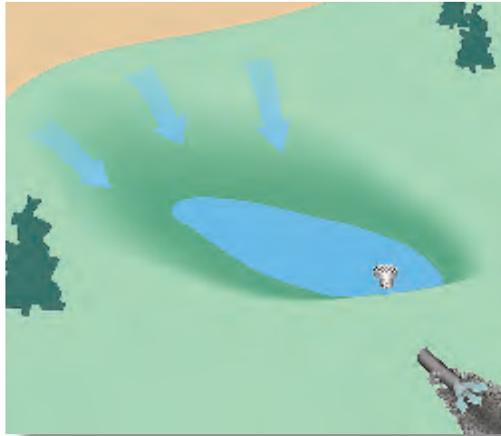
For best results, seed basin sidewalls and upland drainage areas as soon as possible. Make sure outlet structure does not allow rapid flow through the basin—use a rock berm, filter fabric, or other means to maximize ponding and detention time.
