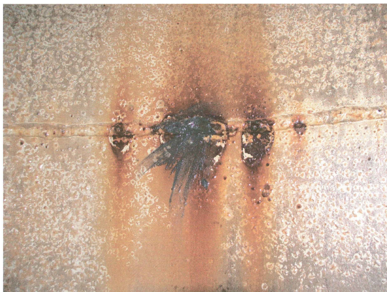
Photo shows an active corrosion cell in the upper section of the riser pipe. The coating in the riser has started to blister.
