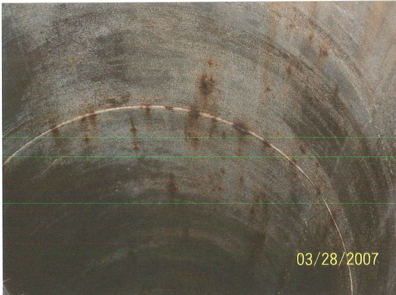
Photo shows the upper section of the riser pipe. Scattered rust nodules cover many surfaces. Corrosion is heaviest along the weld seams.
