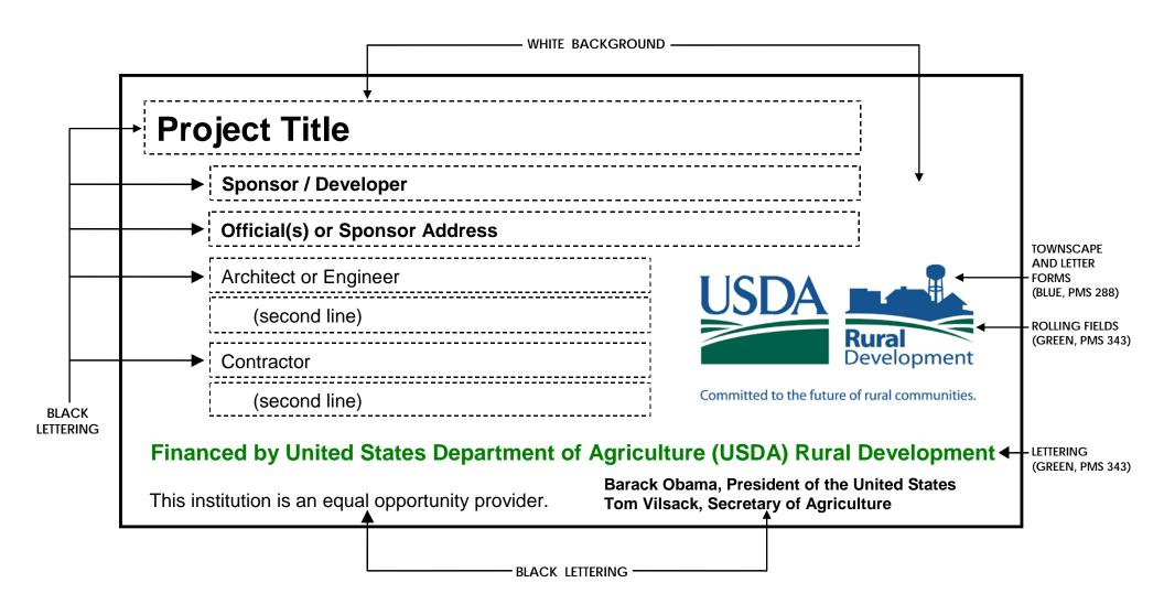
SIGN DIMENSIONS: 1200 mm x 2400 mm x 19 mm (approx. 4' x 8' x 3/4") PLYWOOD PANEL (APA RATED A-B GRADE-EXTERIOR)
