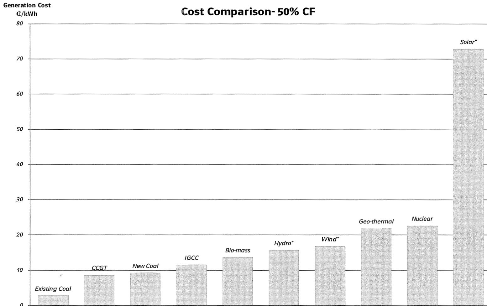
\*Reflects cost of additional capacity required to meet a 50% capacity factor
