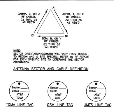
TO PROVIDE ADDITIONAL IDENTIFICATION EACH RF CABLE SHALL BE IDENTIFIED WITH A METAL TAG MADE OF STAINLESS STEEL OR BRASS AND STAMPED WITH THE SECTOR, CABLE NUMBER, AND "AT&T" TO IDENTIFY AT&T MOBILITY CABLES. THE ID MARKING LOCATIONS SHOULD BE AS PER "CABLE MARKING LOCATIONS TABLE". THE TAG SHOULD BE ATTACHED WITH CORROSION PROOF WIRE AROUND THE CABLE. PEFERRED TAG LABELING SHOULD BE AS SHOWN ABOVE "TOMA LINE TAG", "GSM LINE TAG" AND "UMTS LINE TAG".
