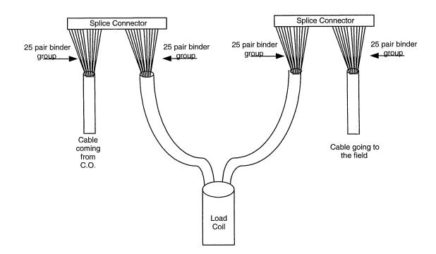
Splicing Example 2 - Load Coil
