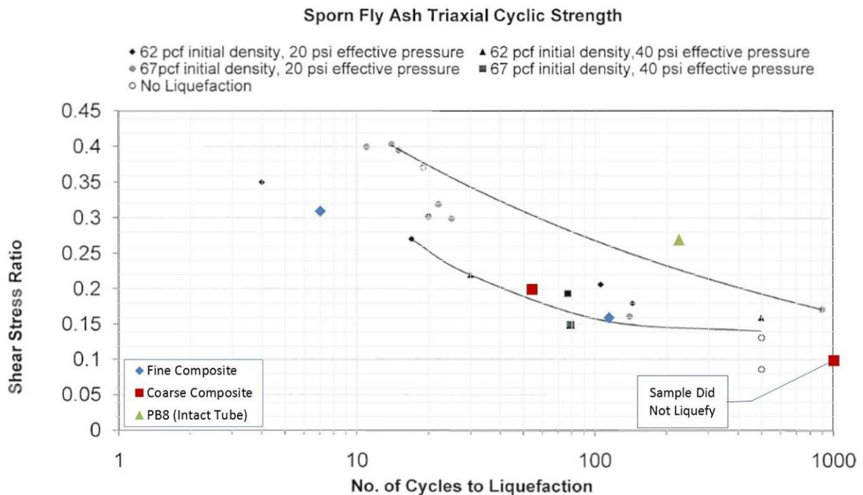
It is observed that the results for reconstituted samples generally fall within but toward the lower end of the band for the Sporn data. The undisturbed specimen plots well above the band from the Sporn data. Resonant column testing was performed on two reconstituted samples – one fine and one coarse. The results of the resonant column testing are depicted in the figure below:
