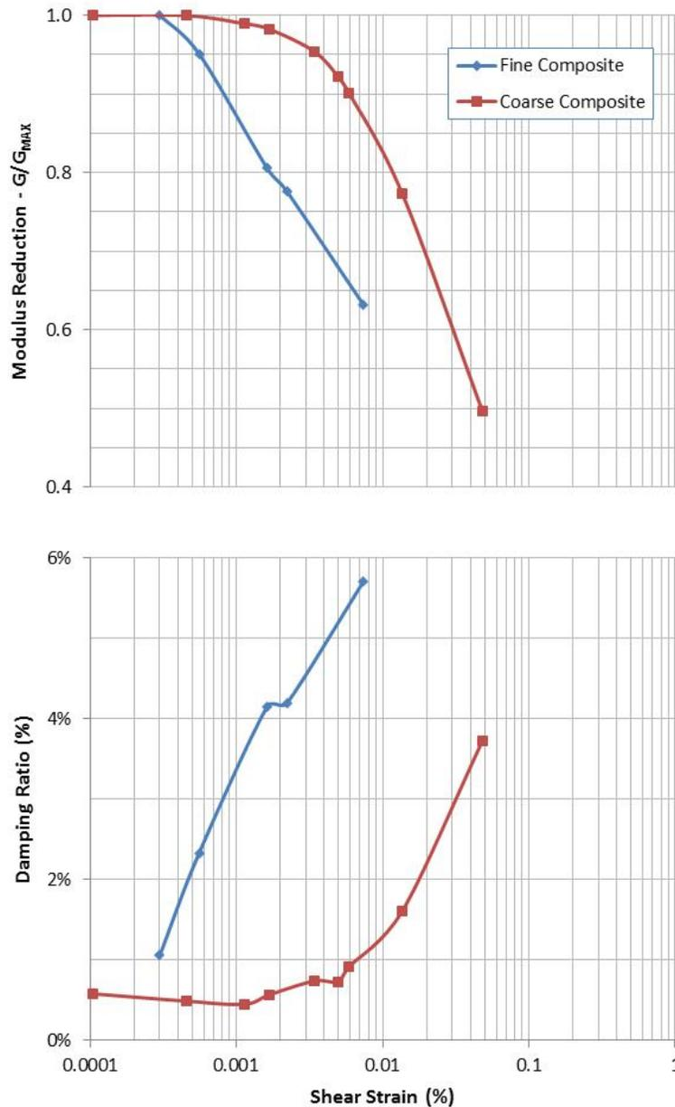
The results of the resonant column testing for the fine composite sample do not plot well or agree with the coarse composite specimen results. This may represent an issue with the fine specimen or the testing itself, and it is recommended that the fine results not be relied upon for performing detailed analyses.
