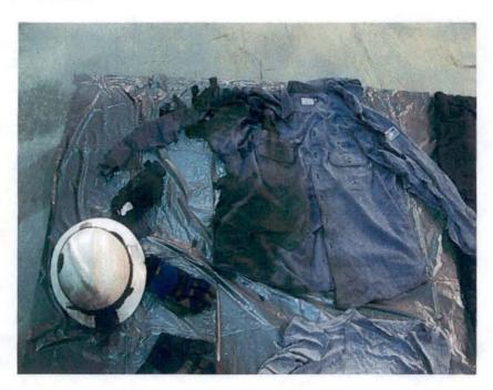
Photo 7. Maintenance Electrician A's clothes. Note burns to right side of body.
