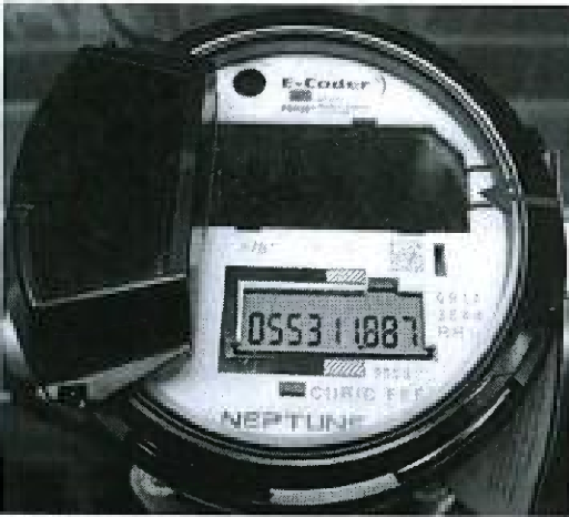
Cubic Feet E-Coder. The solar panel supplies the power to light up the display.
