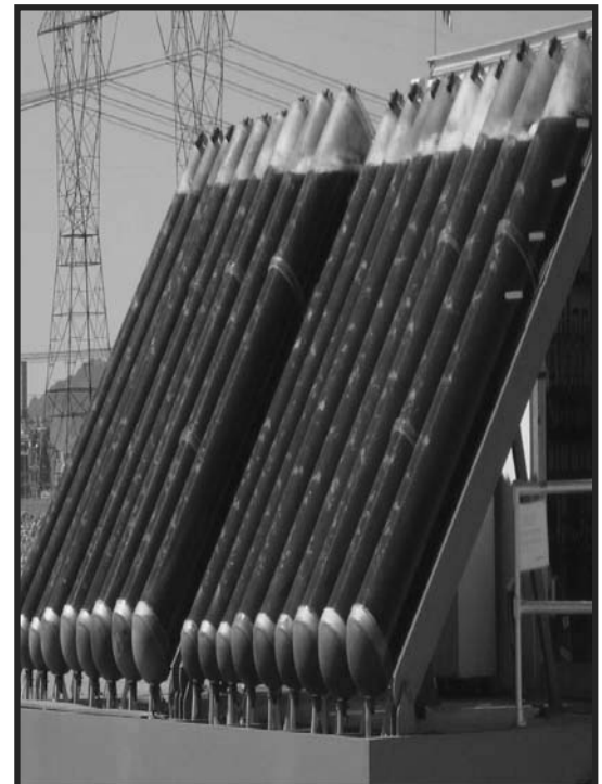
Figure 22: Arizona Public Services' Redhawk power station where algae is harvested and used to produce biodiesel. (Image provided by Raymond Hobbs, APS Senior Engineer, at the Illinois Basin Energy Conference, held March 6, 2008, in Henderson, KY.)
